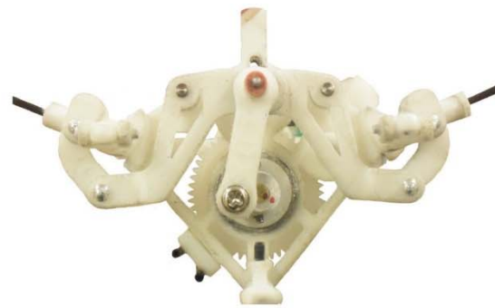
Slider-crank and four-bar mechanism
