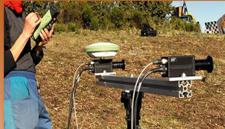
GPS Leica Viva CS10 receptor with RTK system
