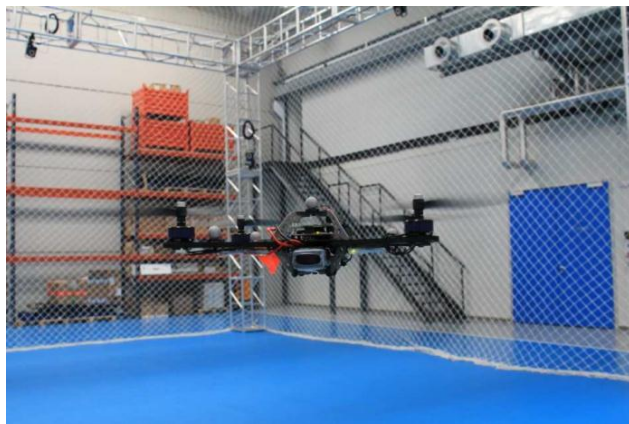
Two UAVs with cameras estimate position of a third UAV, experiments in FADA-CATEC indoor testbed.
