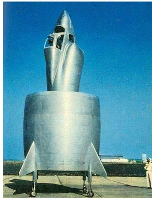
**Annular wing** (aerodynamic lift, symmetry about thrust direction)
